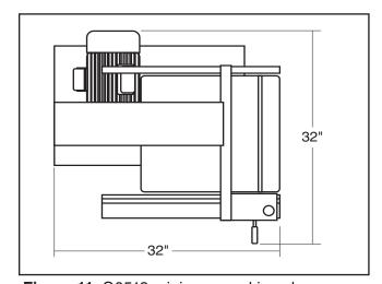
Figure 11. G0513 minimum working clearances.
